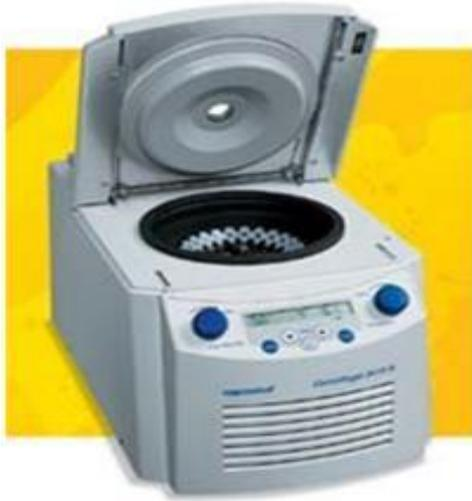
A *centrifuge* such as this can spin at up to 15,000 rpm to facilitate separation of the different phases of the extraction. It is also used to precipitate the DNA after the salts are washed away with ethanol and or isopropanol.
