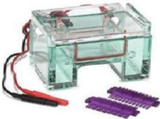
A *gel box* is used to separate DNA in an the net negative charge of the molecule. Different sized pieces of DNA move at different rates, with the larger pieces moving more slowly through the porous medium, thereby creating a size separation that can be differentiated in a gel.
