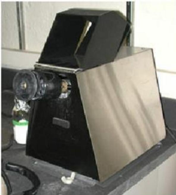
This *bead beater* is used in the breaking apart or "lysing" of cells in the early steps of extraction in order to make the DNA accessible. Glass beads are added to an eppendorph tube containing a sample of interest and the bead beater vigorously vibrates the solution causing the glass beads to physically break apart the cells. Other methods used for lysing cells include a french press and a sonication device.
